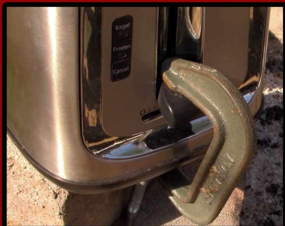
Figure 3. Toaster clamped for SPT combustion
